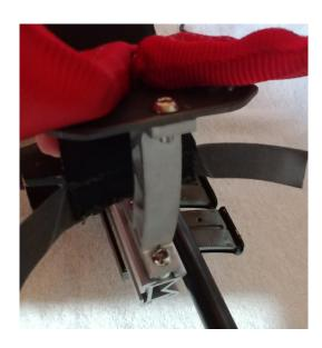
1-Place the pad on the rifle underneath the harness bracket with the hook & loop wings towards the bracket and start to wrap the wings around the sides of the bracket
