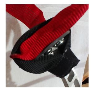
2-Fold the bottom end of the pad up over the front of the bracket plate and ends of the shoulder strap and wrap the hook & loop wings around the bottom end of the pad, basically you are wrapping the bracket plate up inside the pad.
